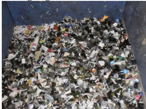
Glass fines bin
